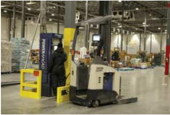
An employee in the Perishables DC fills up a hydrogen-powered forklift. The entire material handling fleet uses hydrogen fuel cells. (Jason McNamara photo)
